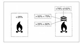
Indication of faults The room unit indicates faults that may have occurred in the unit itself or in the system
