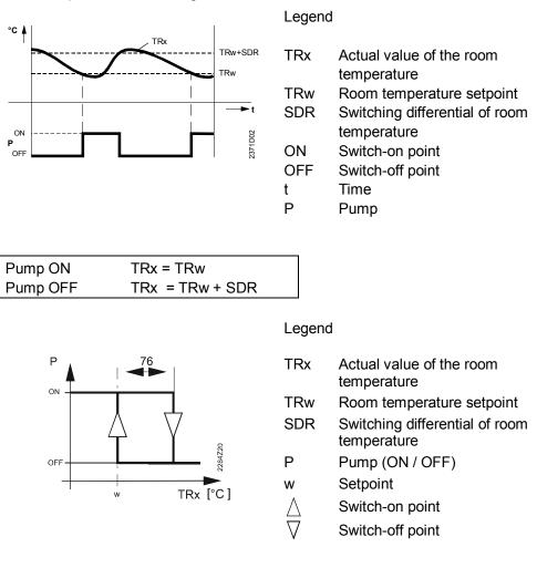
Note The heating circuit pumps are controlled not directly by the QAA73.110, but by boiler control. For this reason, this functionality is not ensured by the room unit alone.
