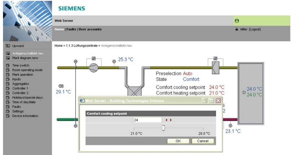
Users can also embed additional data in a plant diagram such as links to plant, function and maintenance descriptions or data sheets. Moreover, users can integrate external links allowing, for example, to directly browse multiple plants. Users can even embed current webcam images in a plant diagram.
